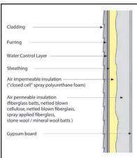
Figure 3: Hybrid walls can be constructed where spray polyurethane foam can be used in conjunction with other cavity insulations such as fiberglass and cellulose.
