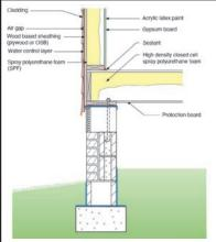
Figure 14: A protection board such as fibercement should be installed to prevent animals from getting into the floor assembly.
