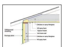
Figure 8: Vented unconditioned attics are typically constructed using spray foam in conjunction with fiberglass or cellulose insulation. The key to the performance of vented unconditioned attics is continuity of the air control layer located at the ceiling plane.
