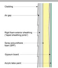
Notes: High density closed cell foam can be used in all IECC Climate Zones. Where low density open cell foam can be used the thickness or thermal resistance of the rigid foam exterior sheathing is specified by the International Residential Code (IRC) based on Climate Zone and the thickness of the wall framing.
